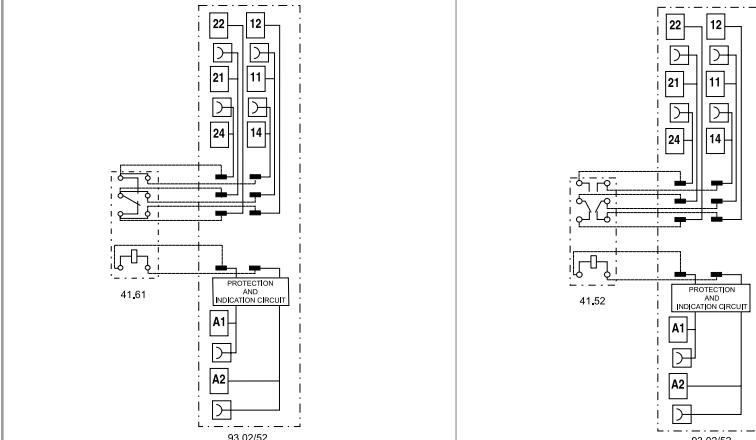
\* For currents > 10 A, contact terminals must be connected in parallel (21 with 11, 24 with 14, 22 with 12).
