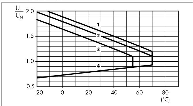
1 - Max. permitted coil voltage at nominal load (DC coil).
