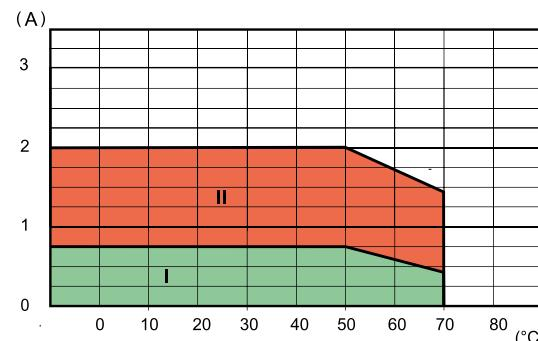
I: SSR installed as a group (without gap between sockets)
