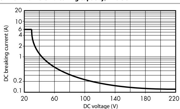
H 38 - Maximum DC1 breaking capacity, 1 Pole 16 A and 2 Pole 8 A
