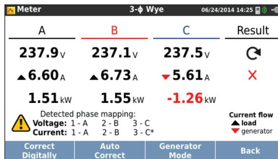
Intelligent verification function that digitally corrects most common measurement connections
